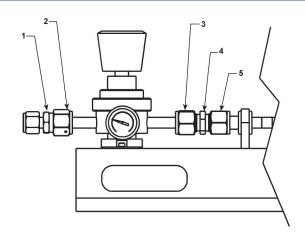
Figure 1. 1/2 in. molstic-S, with Back Pressure Regulator
